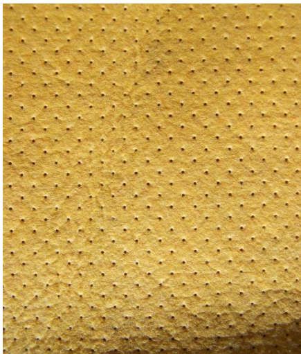
Fig. 14. Polypropylene and cotton filter
